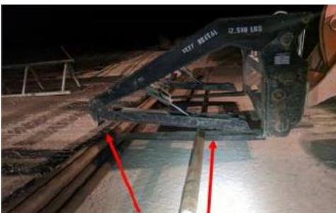
The position and number of the pipe does not allow grapple clamp to compress on all the joints resulting in an opening at the end of the fork tines greater than pipe circumference.
