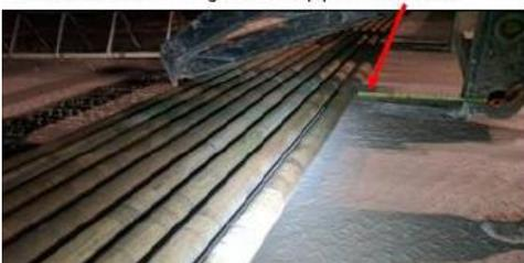
While moving 9 joints of 33' 4" drill pipe weighing approximately 462lbs per joint between pipe racks with the pipe grapple system engaged, the pipe became free from the grapple, causing 8 of them to descend approximately 6ft to the ground.
