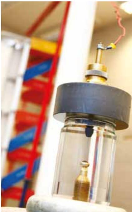
**FIGURE 2:** The needle-sphere electrode configuration used for lightning impulse breakdown testing.
