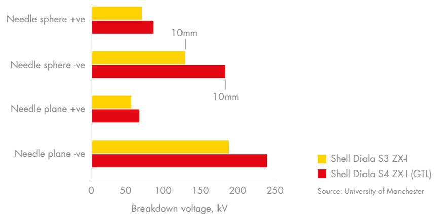
**FIGURE 3:** Average lightning impulse breakdown voltage of inhibited GTL oil (Shell Diala S4 ZX-I) versus conventional inhibited oil (Shell Diala S3 ZX-I) with a 25-mm electrode gap, unless otherwise specified.
