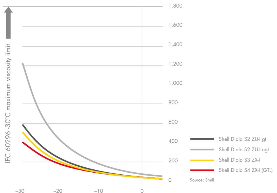
**FIGURE 5:** Fluidity (viscosity, cSt) versus temperature (°C) for inhibited GTL transformer oil (Shell Diala S4 ZX-I) compared with conventional oils: uninhibited (Shell Diala S2 ZU-I ngt) and inhibited (Shell Diala S3 ZX-I).
