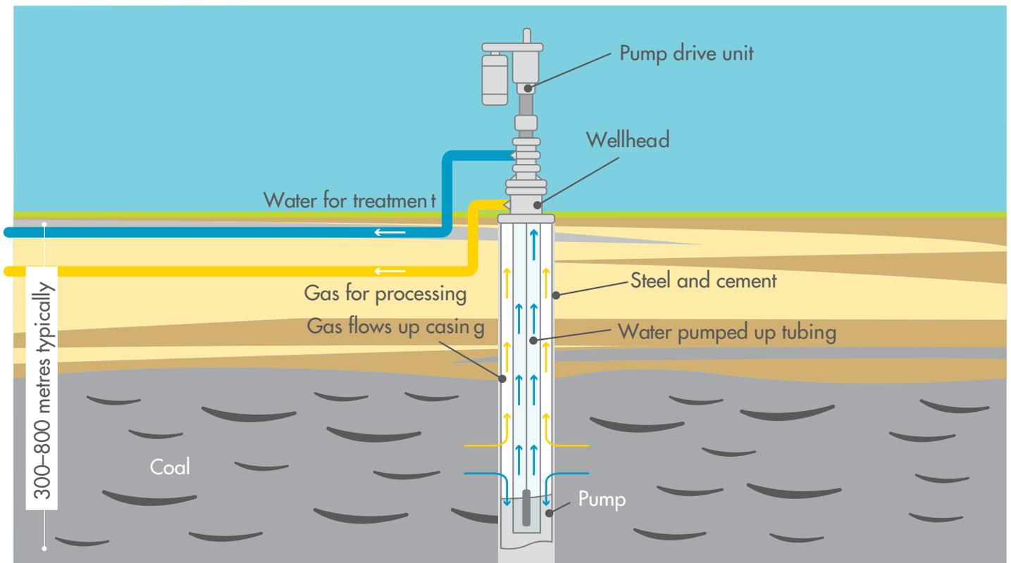
Wells are designed and built using steel piping and cement. These barriers seal the well to prevent the flow of liquids or gases from the coal seam into other formations.
