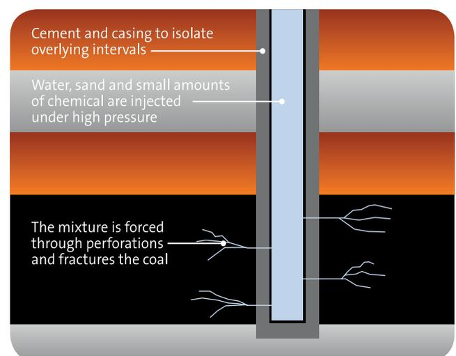
High-pressure pumps inject the fracturing fluid back into wells to open tiny cracks in the coal seam.
