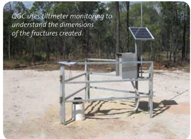
*QGC uses tilmeter monitoring to understand the dimensions of the fractures created.*
