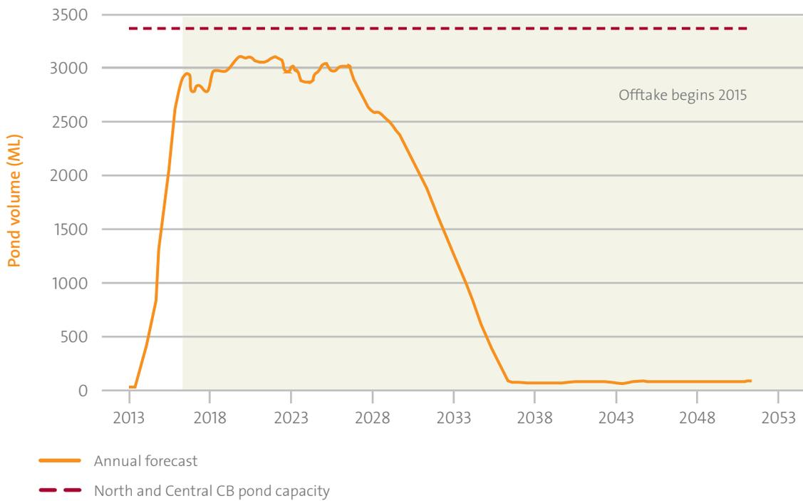
Figure 15-14 – CWTP and NWTP Concentrated Brine Pond volume and capacity
