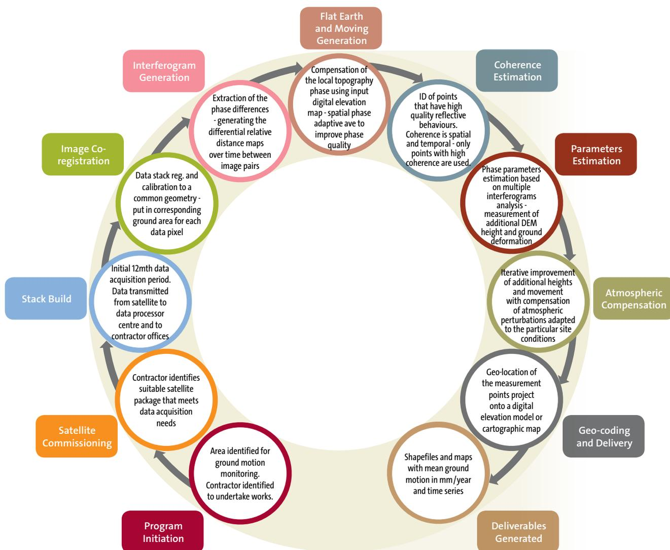
Figure 10-2 – Ground motion data acquisition and processing
