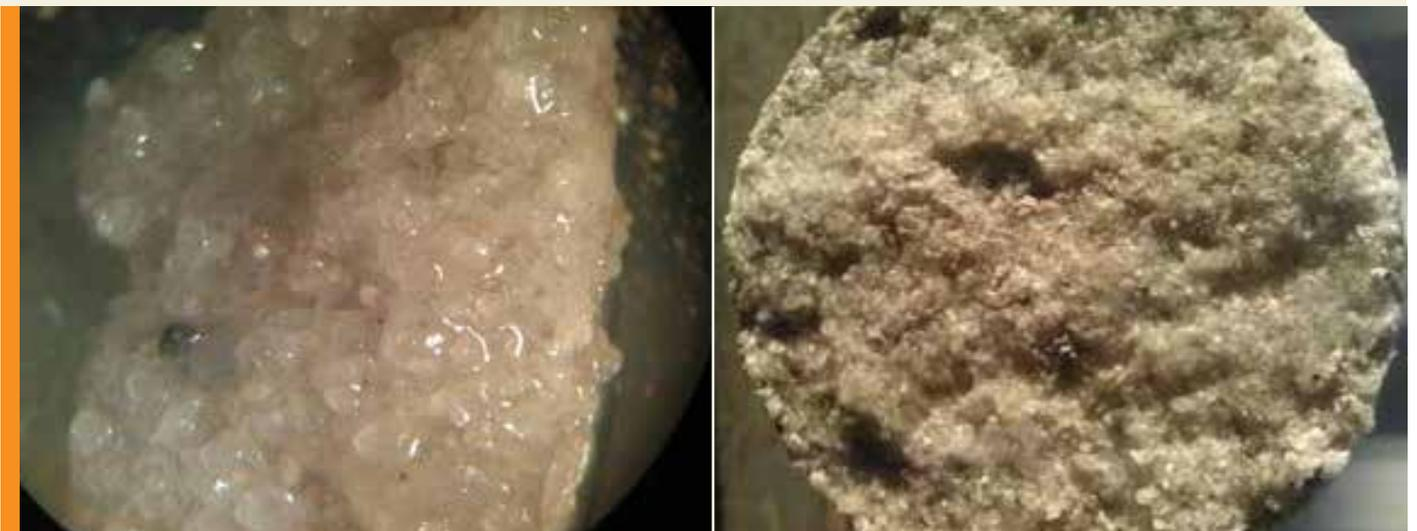
Figure 40 – Precipice Sandstone core from Monitoring Bore GW4 Woleebee Creek
