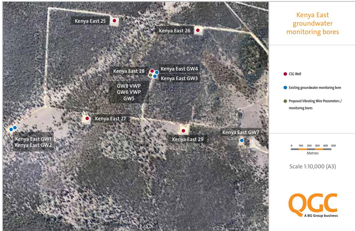
Figure 28 – Kenya East P3 pilot groundwater monitoring bores layout
