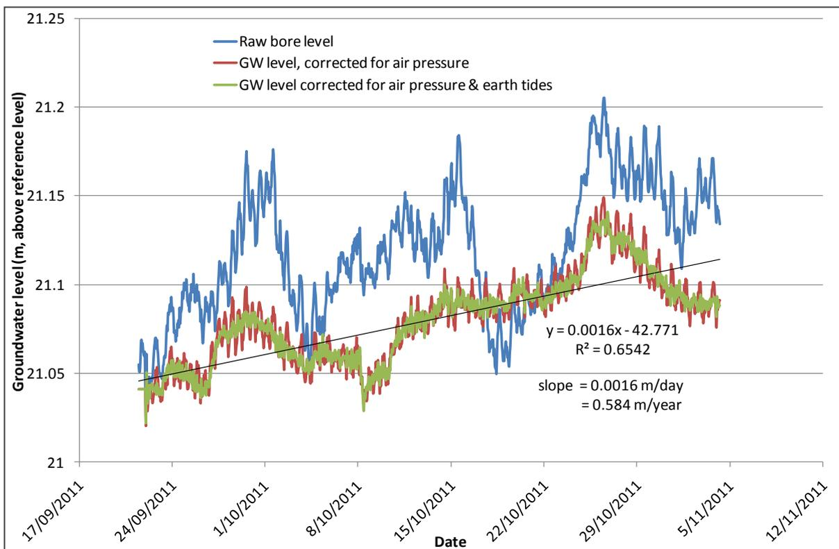
Figure 4: Groundwater level accounting for air pressure and earth tides
