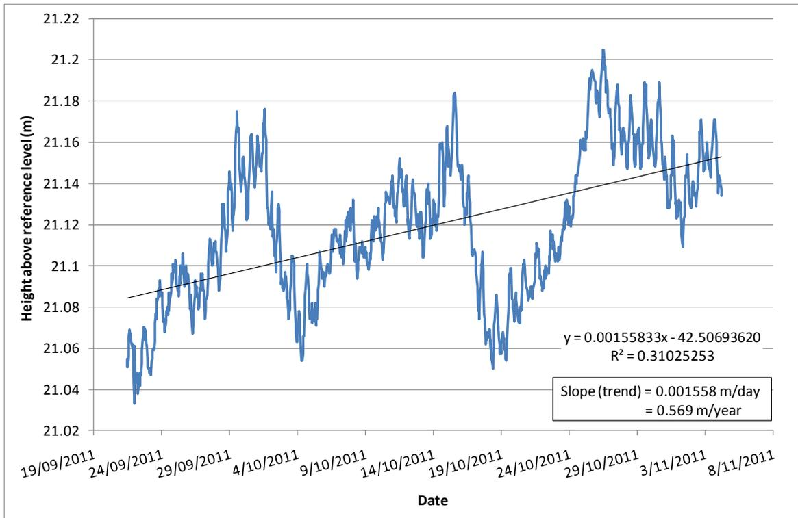
**Figure 2: Groundwater level time series and linear trend for Berwyndale South GW1**
