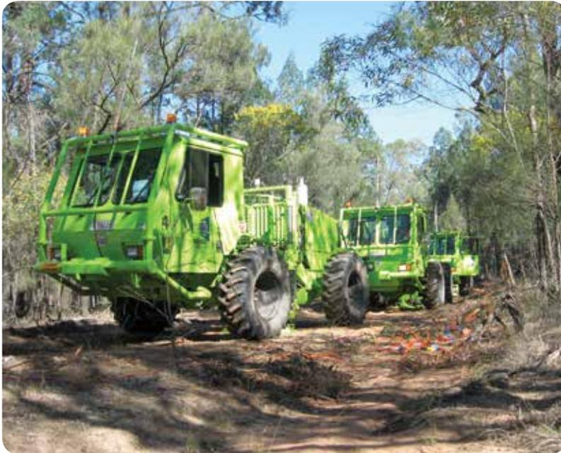
*Vibroseis trucks send acoustic waves into the earth. A recording truck is connected to up to 10km of cable to receive the seismic signal*
