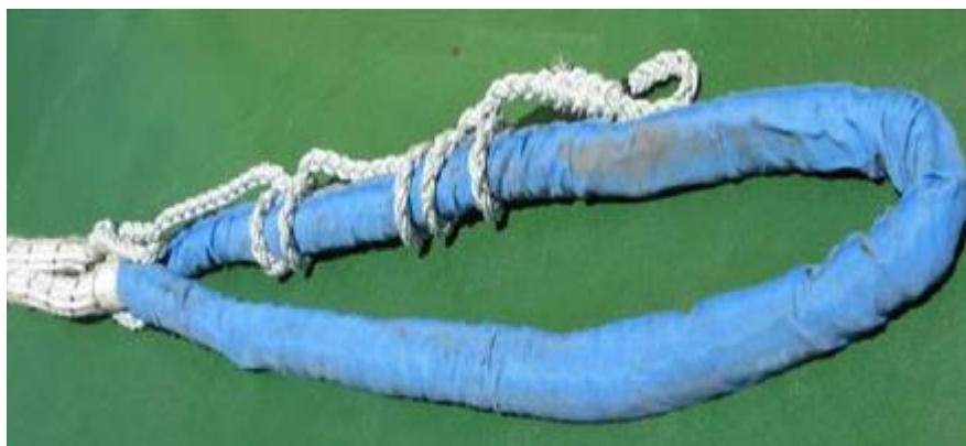
Figure 7: Mooring tail / pennant fitted with Jockey Rope
